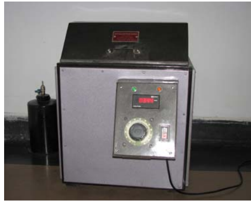
SPECIALLY DESIGNED CRUSHING UNIT FOR RESIDUAL GAS MEASUREMENT
